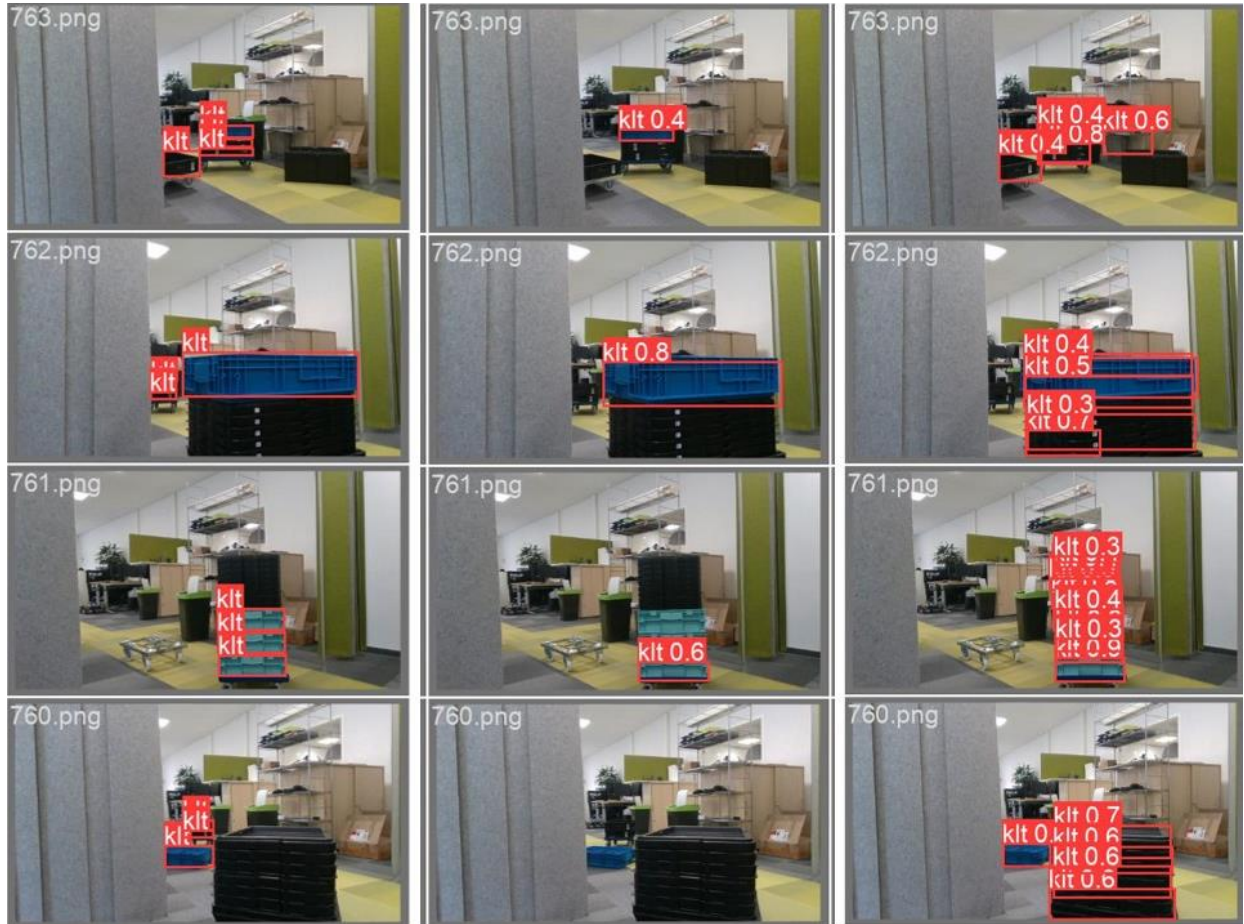
Figure 5.3 YOLOv5s being tested on a real-world environment. On the left, the ground-truth label is shown; on the middle, the Color Light randomization was used for training purposes; and on the right the HDRI randomization approach was followed.
