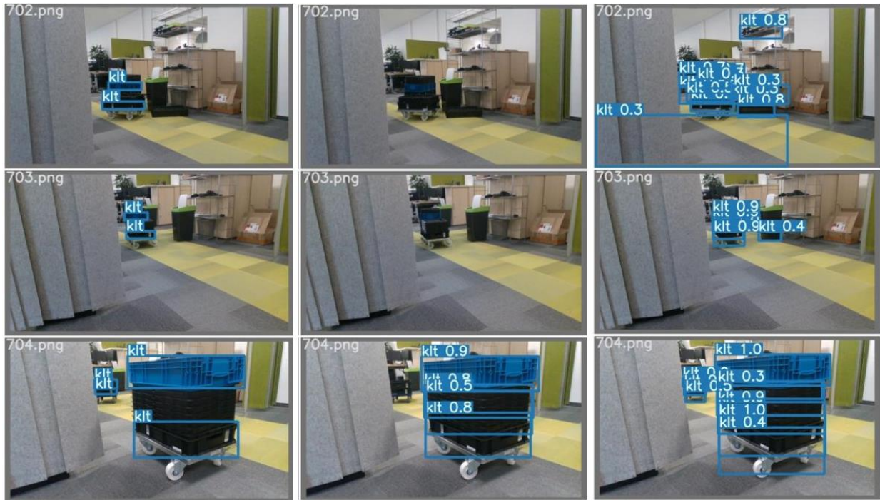
Figure 5.5 YOLOv7 being tested on a real-world environment. On the left, the ground-truth label is shown; on the middle, the Color Light randomization was used for training purposes; and on the right the HDRi randomization approach was followed.
